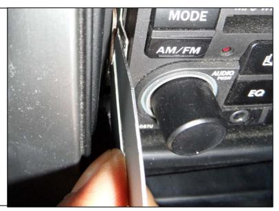
4. Push the tool into the gap until the edge of the tool is hard up and square against the radio front panel as shown. Repeat steps 3 and 4 for the opposite side of the radio.
