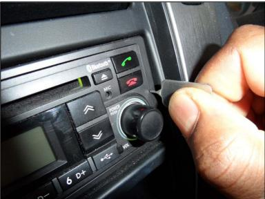
3. Insert the radio removal tool tapered edge into the gap between radio clip and the mounting frame as shown.
