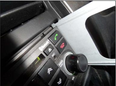
5. Grasp each tool with each hand. Pull the tools outward from the dash equally so that the radio is released approximately 80 mm from the mounting frame as shown. Remove the tools from the radio sides.
