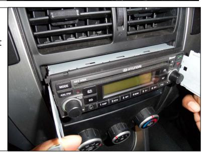
6. Pull the radio out of the dash as shown to reveal the radio rear wiring connectors.
